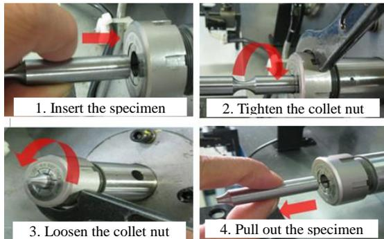
Fig. 4: Simple procedure to fix and remove the specimen
