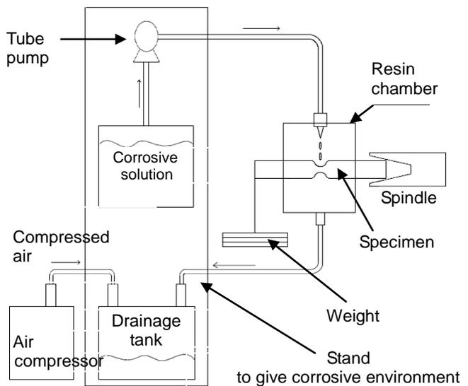
Fig. 7: Schematics of corrosion fatigue testing machine
