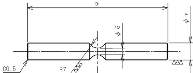
Fig. 3: The shape and dimensions of the specimen
