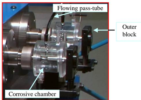
Fig. 6: Corrosive chamber
