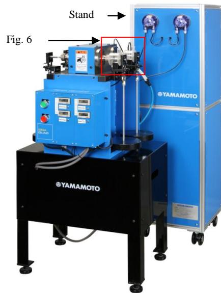
Fig. 5: Photograph of fatigue testing machine combined with the corrosive chamber
